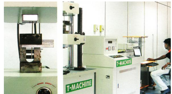
Weld Strength Testing of EsyFence™
